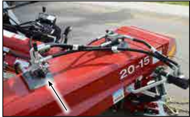
Fig 16 - Hydraulic selector valve
