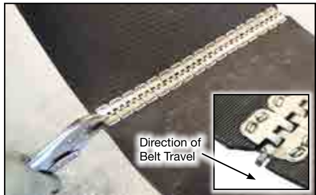
Fig 32 - Crimp lacing and taper belt corners
