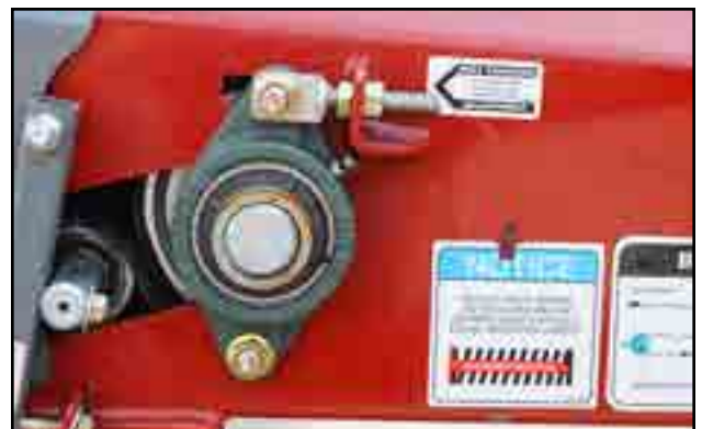
Fig 27 - Conveyor belt adjustment
